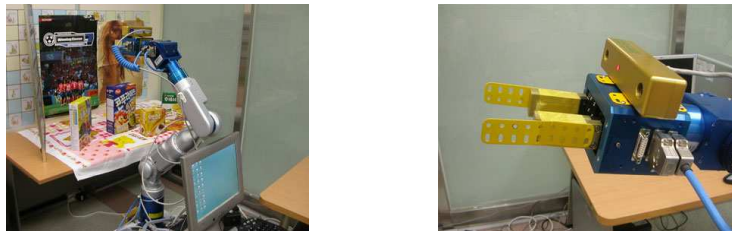
Fig. 1. Experimental environment with an eye-on-hand configuration
