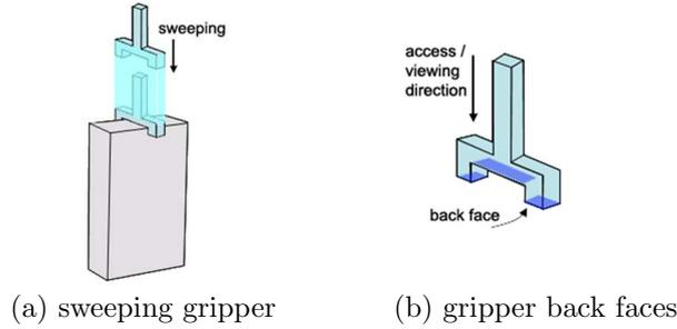
Figure 5: Gripper visibility test with back faces
